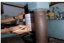
Figure 4: Testing on the samples for Compressive Stress Evaluation
