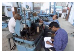
Figure 4: Testing on the samples for Compressive Stress Evaluation
